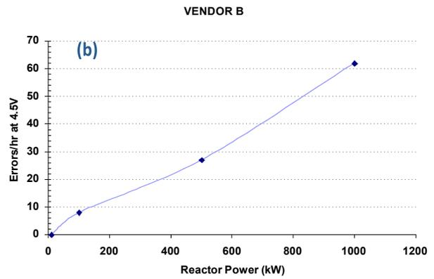
FIGURE 4: The effect of thermal neutron flux on the SER for (a) a 16-kbit memory chip from Vendor A and (b) a 4-Mbit chip from Vendor B
