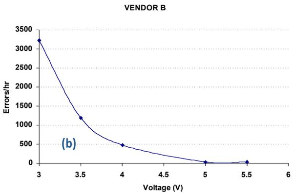
FIGURE 3: The effect of supply voltage on soft errors in (a) a 16-kbit memory chip from Vendor A and (b) a 4-Mbit chip from Vendor B
