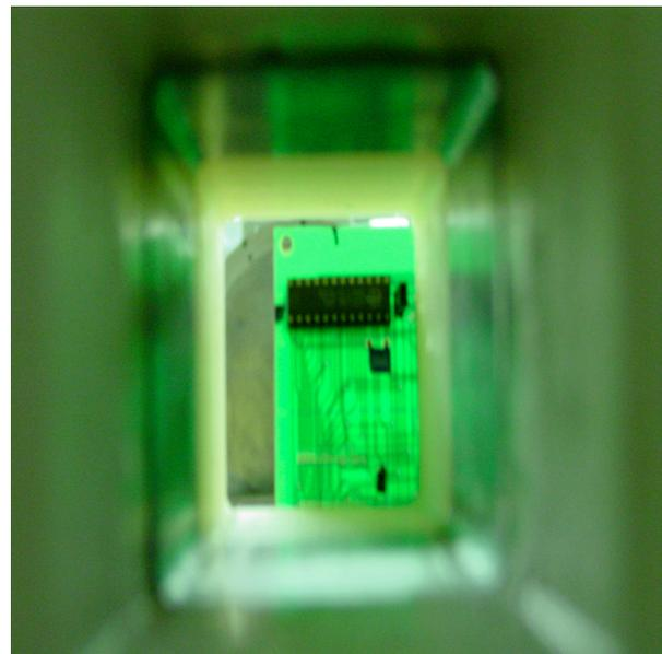
**FIGURE 1:** The experimental test chip, as seen through the narrow opening in the polyethylene/lead shield.
